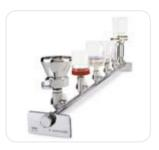
Made of high-grade stainless steel (B.S. 304S3 | AISI 304); accommodates any type of vacuum funnel. Stainless steel three-way valves (taps) allow the vacuum for each filter holder to be individually controlled and each holder to be sterilely vented. The low height of the manifold ports is particularly advantageous for working on a clean bench.
